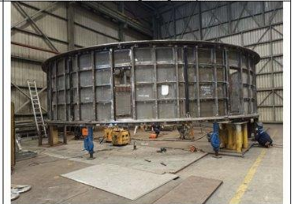
Slipring inner ring ready for painting
